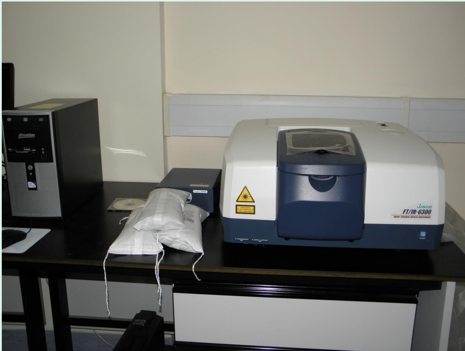
JASCO 6300 FTIR spectrometer ( 350\text{--}7800\text{ cm}^{-1} , 0.07\text{ cm}^{-1} resolution, ATR accessory)
