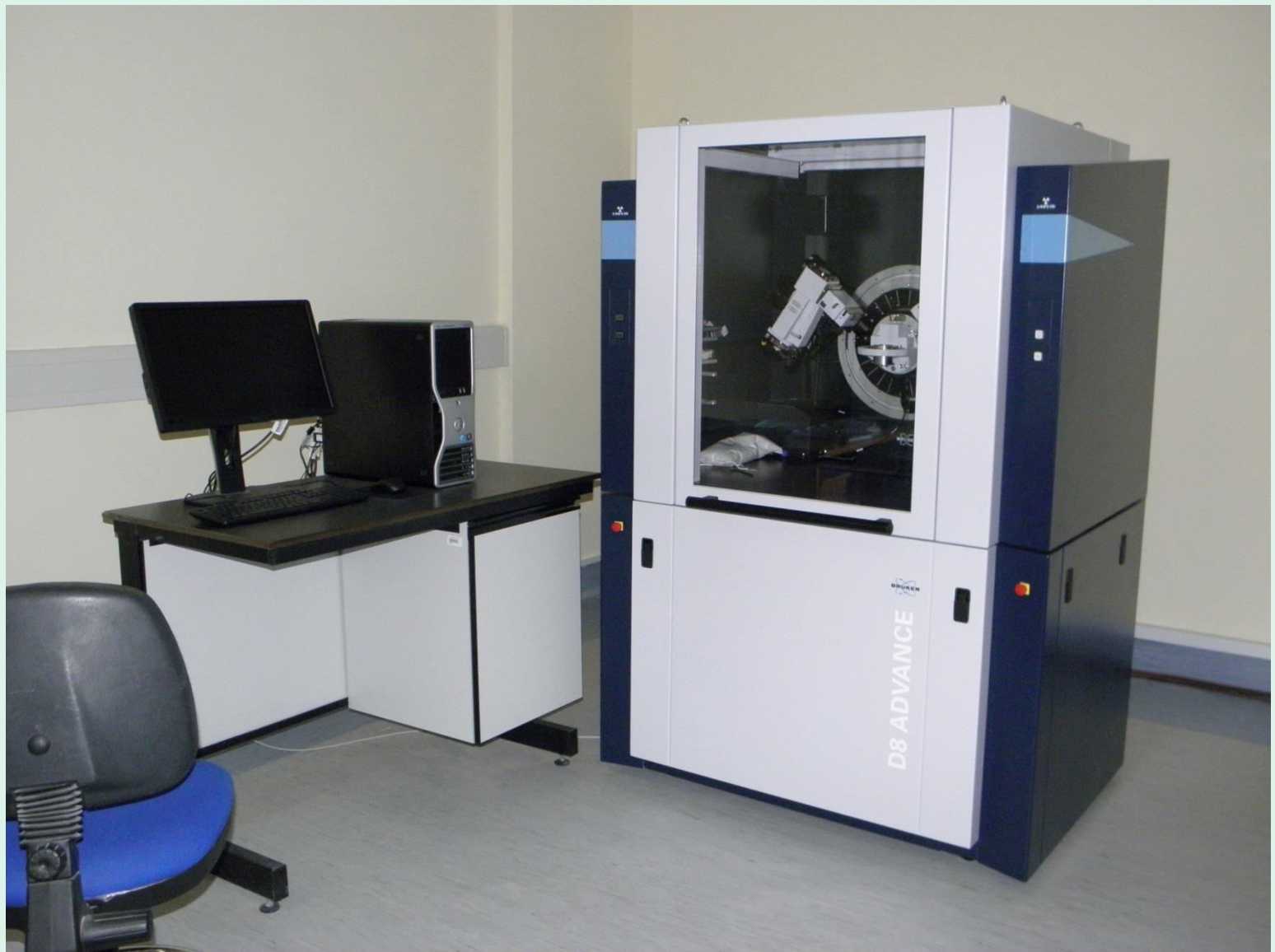
Bruker D8 ADVANCE powder XRD system (2.2 kW Cu tube, point detector)
