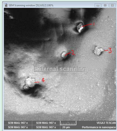
SEM Micrographs: cutoff diameters: 16, 8 µm; X1000
